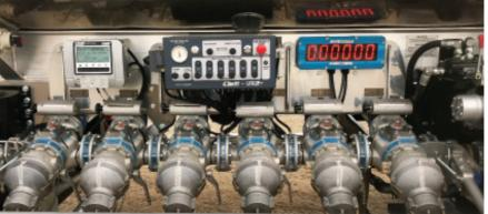
Swift uses level gauging to accurately and conveniently deliver multiple products through a single pump to selectable outlets.
