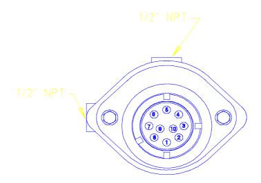
a) Set multimeter to read resistance, range up to 4,000.00 Ω. Hold red lead on No.10 contact and in turn hold the black lead onto contacts numbers 3, 4, 5, 6, etc in turn (assuming all compartments have thermistor probes). The meter should read on average 2000 Ω. On a hot day (30°C): Approximately between 1000-1500 Ω. On a cold day (10°): Approximately 2500-3500 Ω.
